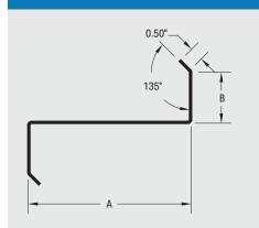
Material Thickness: 12, 14, 16 gauge "A" Dimension: 6.0", 6.5", 7.0" "B" Dimension: 1.87," 2.0," 3.0," 3.5," 4.0"
